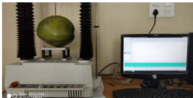
Fig. 7. Texture analyser test for punching energy requirement study
