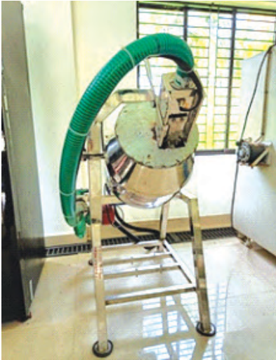
Fig. 123. Rotary dryer-cum-flavour coating machine
