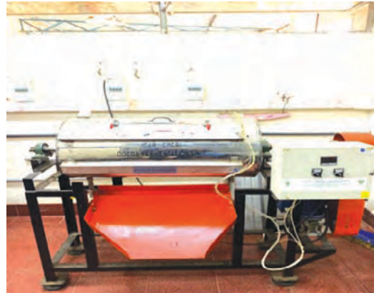
Fig. 124. Cocoa bean fermenter device
