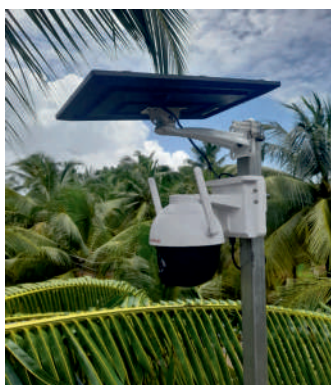
Fig. 44. Camera installed to monitor the activity of pollinators and insect pests
