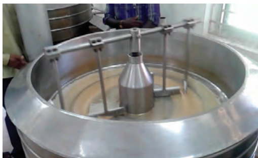
Fig 15. Double jacketed cooker for processing Kalparasa into sugar, jaggery and honey
