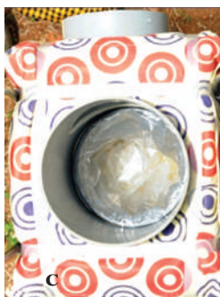
Fig. 8c. Polythene pouch with O-ring fixed above the groove
