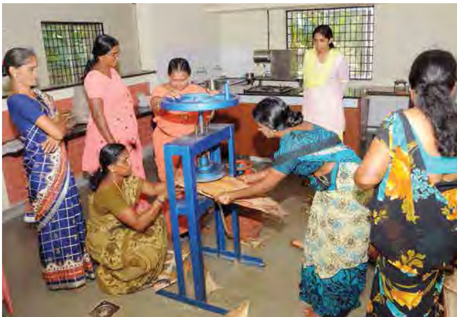
Making eco-friendly plates from areca leaf sheath
