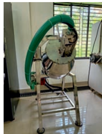
Innovation in motion: rotary dryer-cum-flavour coating for coconut chips
