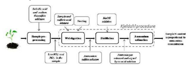
Working Principles: During digestion step all amino-N is converted to ammonical radical.
